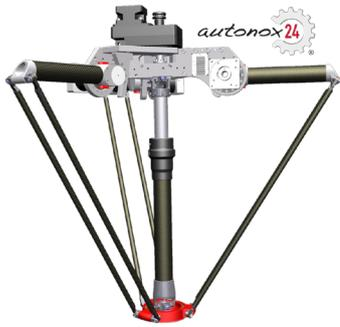
A bestseller in the autonox24-portfolio: The DELTA robot kinematic RL4, designed for a net payload of 6 kilograms.
