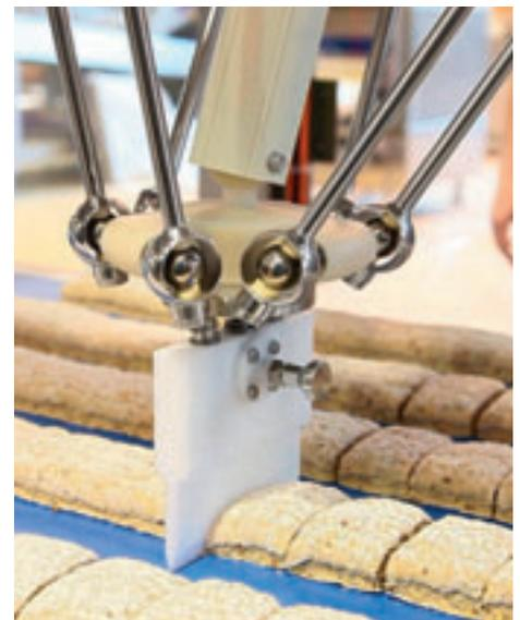
Portioning bread rolls on a moving conveyor belt – precise down to a gram
